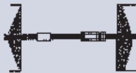
Coupler turnbuckle arrangement for connecting two fixed bars
