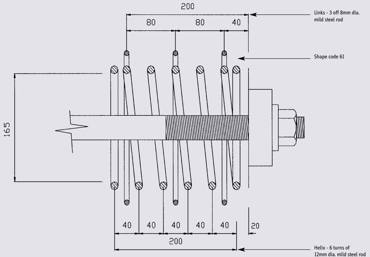
Table 7 Suggested Mild Steel End Block Reinforcement (helix and links must be used together with minimum  $35\text{N/mm}^2$  concrete – see Figure 3)
